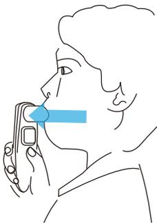
**5** After the readings become visible on the screen, the Peak Flow Meter will transmit the data to the Gateway. If the LED ring is **Green**, you have properly taken a measurement for the day and that measurement has been successfully transmitted. The Peak Flow Meter will automatically shut down.
